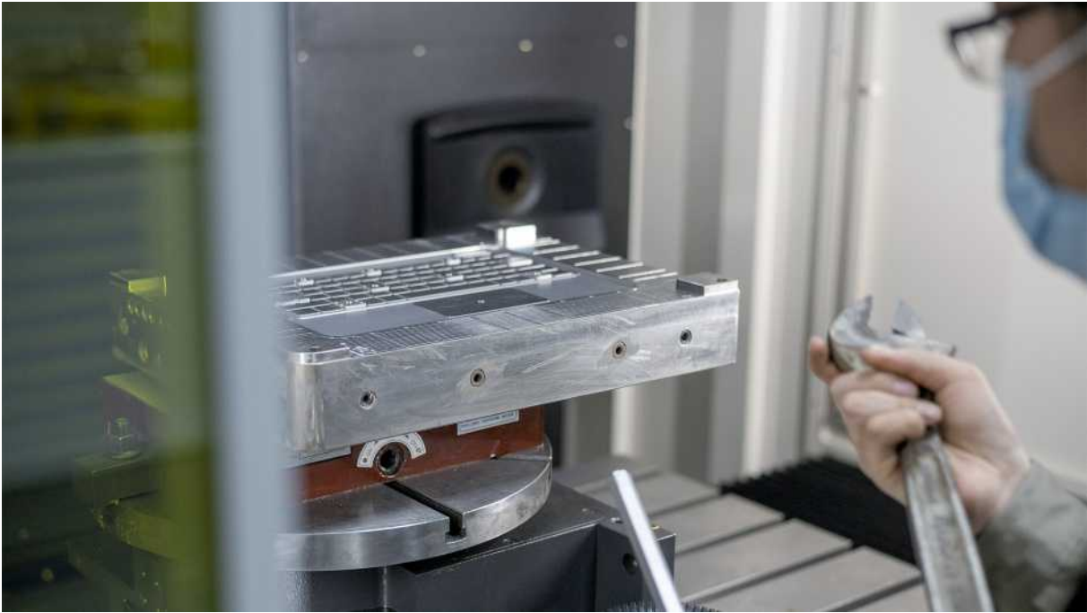
Loading of a laptop mold on the machine table of AgieCharmilles Laser S 1000 U. The laser texturing process starts from here.
