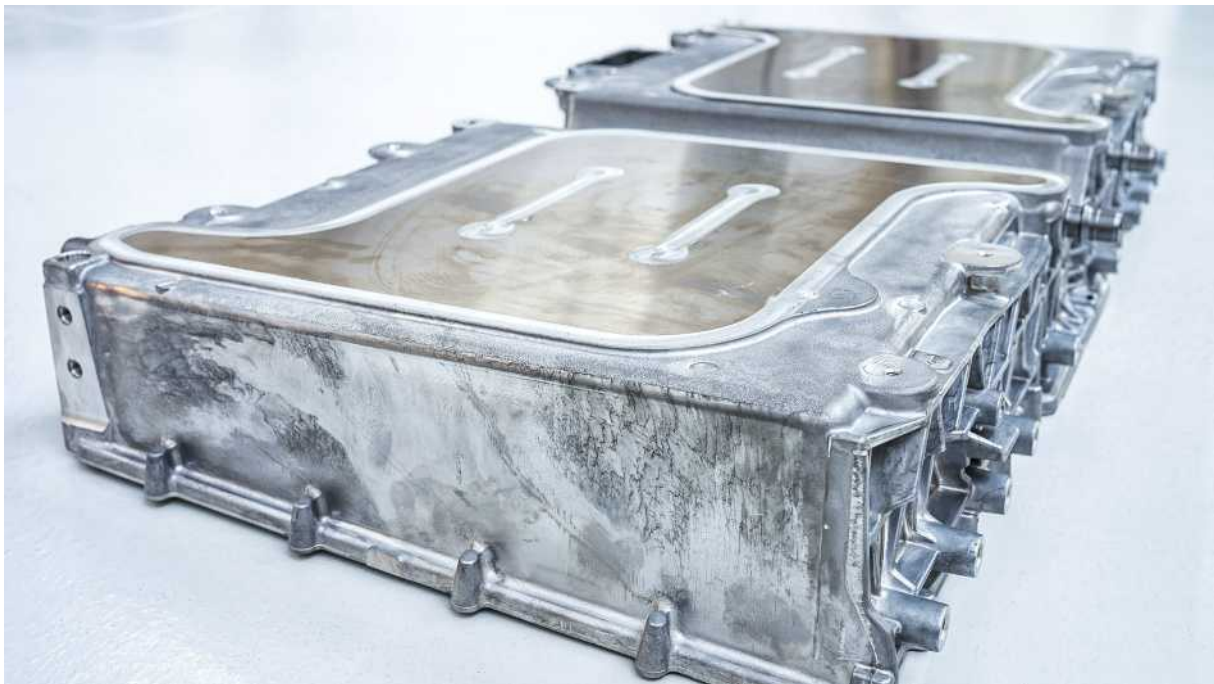
The result of GF Casting Solutions' four years of development work for Renault is the battery housing made of an aluminum alloy measuring 1.00 x 0.55 x 0.15 meters and weighing around 15 kilograms, including cooling circuit covers.
